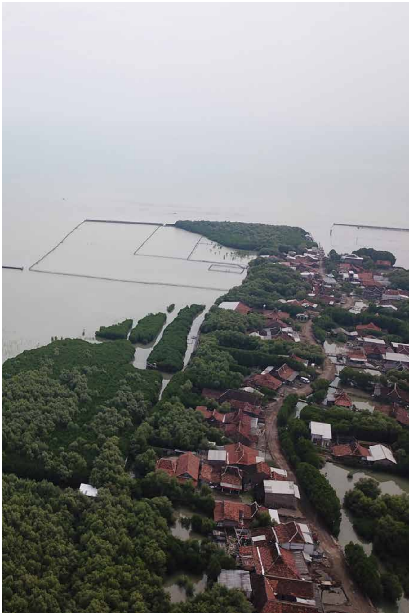
The permeable structures neighbouring the village of Timbulsloko, where the project activities started.
